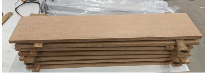
The first thing that will need completed is to mill the rough lumber to workable boards. I have cut all the boards to a more manageable length.
